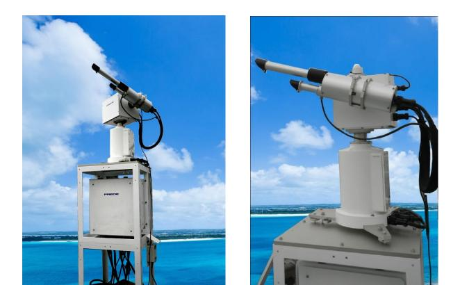
POM-01 MK-III Skyradiometer measures circumsolar radiation and spectrum intensity of the direct solar radiation for the research of the size distribution and concentration of the aerosols. Sensor part is loaded on the sun tracker, and it automatically follows the direction of the sun by the sun sensor.
